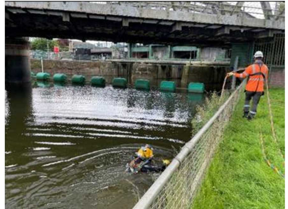
Diver carrying out a survey in the River Witham around the Grand Sluice
