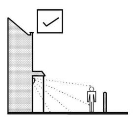
Besides being cheap to run, this type of light is kinder to the night time environment providing a gentle wash of light with reduced glare. Bulkhead and porch lights cast fewer shadows, reducing the hiding places for criminals. These units can also be fitted with a movement detector if required. These units are generally mounted lower and are therefore less susceptible to nuisance switching and complaints from neighbours.
